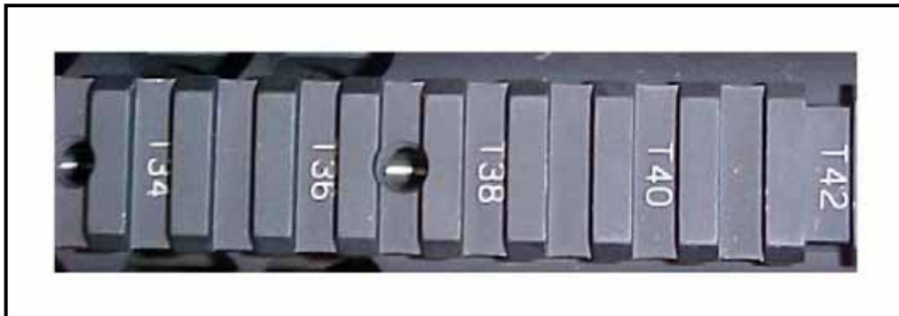
Figure 2-16. Address markings on RAS.
