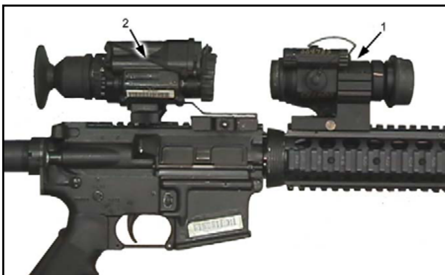
Figure 2-26. Mounting the M68/AN/PVS-14 combination on an MWS.
