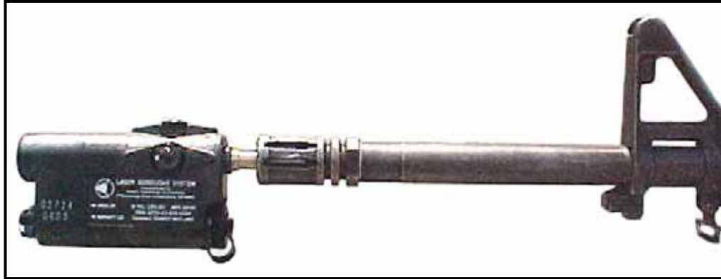
Figure 8-4. Borelight in the HALF TURN position.
