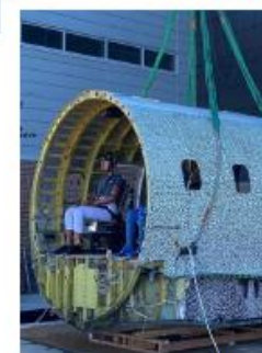
Severe Impact: Fuselage Drop
